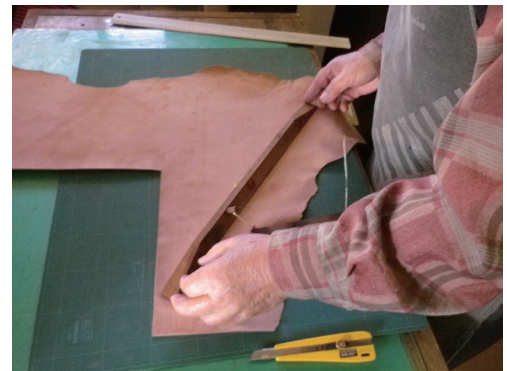
図14 新しい革に貼替え Fig. 14 New leather upholstered to replace the damaged leather
