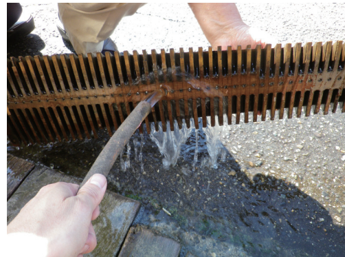
図8 分離後の笛室を水道水で洗う Fig. 8 The wind chest is washed with tap water after separation
