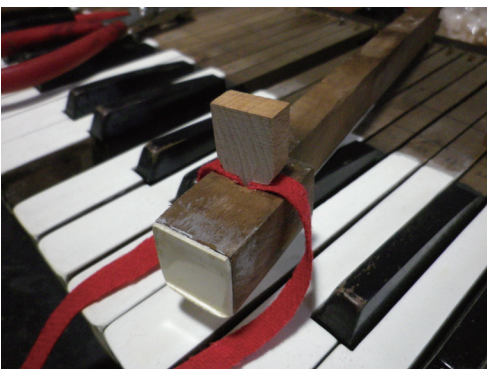
図15 鍵盤裏のクロスも交換 Fig. 15 The cloth behind the keyboard is another component that has been replaced
