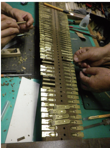
図11 笛室の脆くなった部分を取り除き、新しい木を接着 Fig. 11 New wooden parts are glued to the wind chest after removing the parts that have become brittle
