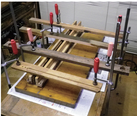
図13 分離した笛室と響板を再接着 Fig. 13 The separated components of the wind chest and sound board are glued together
